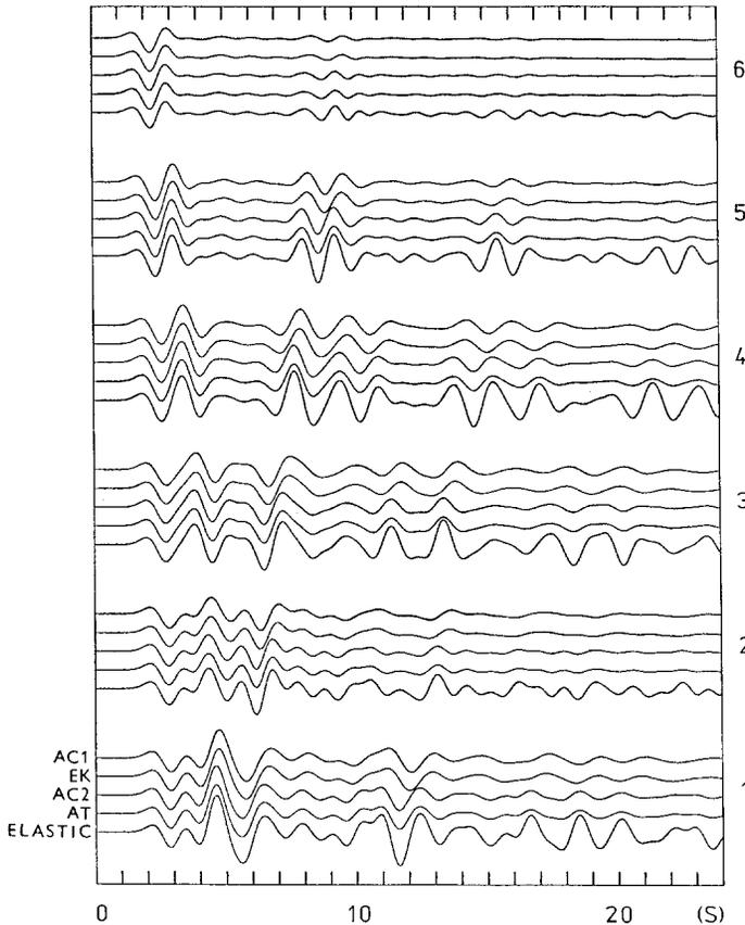
FIG. 2. A comparison of the absorbing-medium response  $p(t)$  computed by four independent methods for six receivers of the basin model in Figure 1. EK and AT: the *reference* solutions for  $\gamma = 0$  and  $\gamma = 1$ , respectively; AC1 and AC2: the *approximate* solutions of this paper for  $\gamma = 0$  and  $\gamma = 1$ , respectively. ELASTIC denotes the perfectly elastic response  $r(t)$ .
