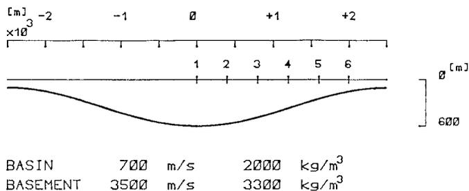
FIG. 1. Model of sedimentary basin used for checking the absorption corrections of the present paper by the finite-difference method in Figure 2. The receivers are denoted by numbers 1 to 6. The shear-wave velocities and densities are also shown.
